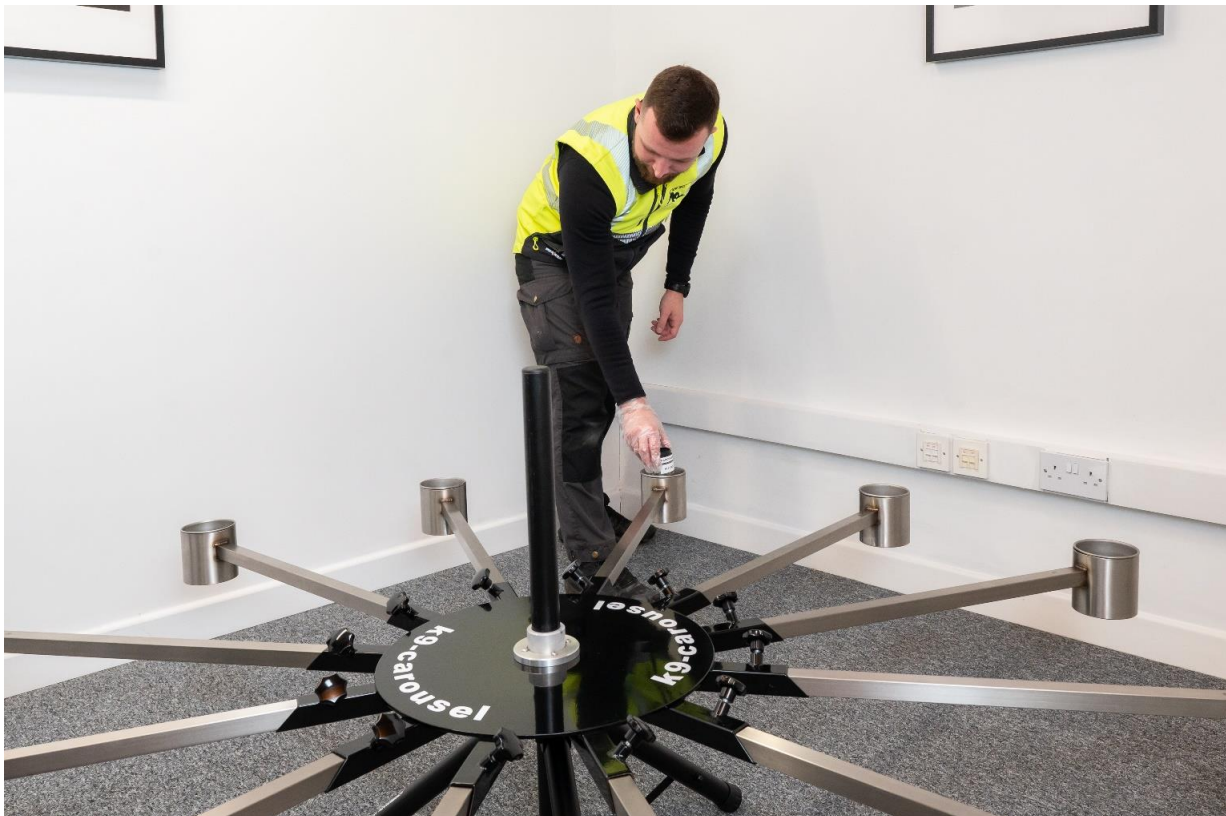
Figure 2: Training carousel being loaded with TADDs prior to training. The carousel can rotate between training runs to prevent the dog relying on special memory of where the target scent was previously located.
