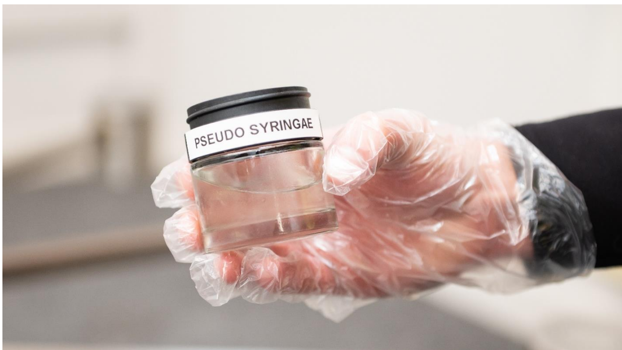
Figure 1: A Target Analyte Detection Devices (TADDs) used to safely store the scent material, there is a filter membrane in the black section to allow scent detection.
